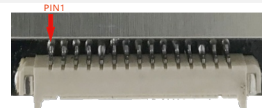
15 PIN W-TO-B 连接器, 1.25mm
